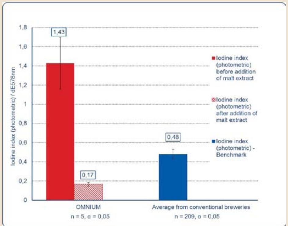
Fig. 1 Photometric measurement of the iodine values before and after dosing the malt extract, benchmarking current industry figures for cold wort according to Research Center Weihenstephan for Brewing and Food Quality, (Analysis with buffered method, standard value < 0.45; MEBAK – Wort, Beer, Beer-based Beverages, Edition 2013, p. 53)
