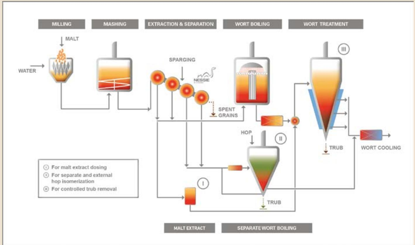
Fig. 2 Schematic illustration of the novel brewhouse concept
