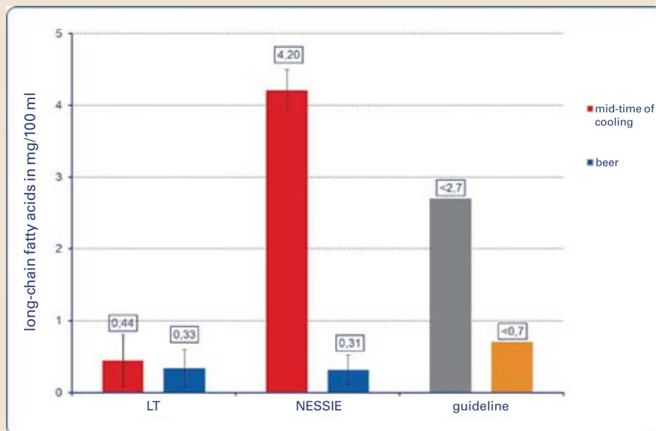
Fig.4 Long-chain fatty acids at half-time of cooling and in beer: palmitic, stearic, oleic, linoleic and linolenic acids (n=2-5,  $\alpha=0.05$ )
