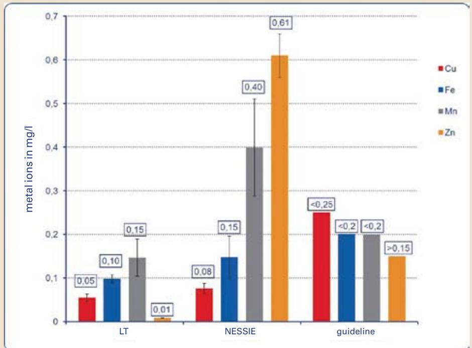
Fig. 3 Metal ions in half-time cooling wort (n=3-5, α=0.05)
