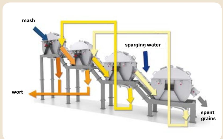
Fig.1 Process diagram of the novel mash filtration system
