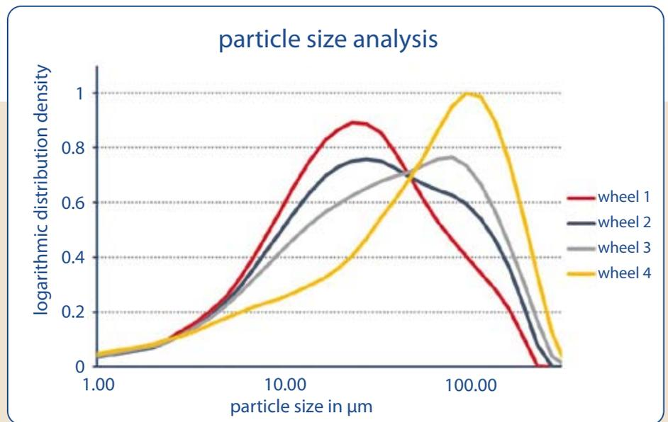
Fig. 2 Logarithmic distribution density of particle size analyses of the novel mash filtration system – wheel 1 to wheel 4
