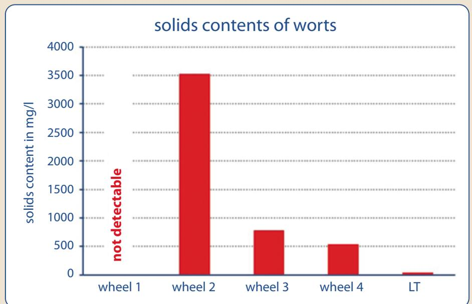
Fig. 3 Solids content of the individual rotary disk filter worts compared to the pfannevoll wort of a lauter tun
