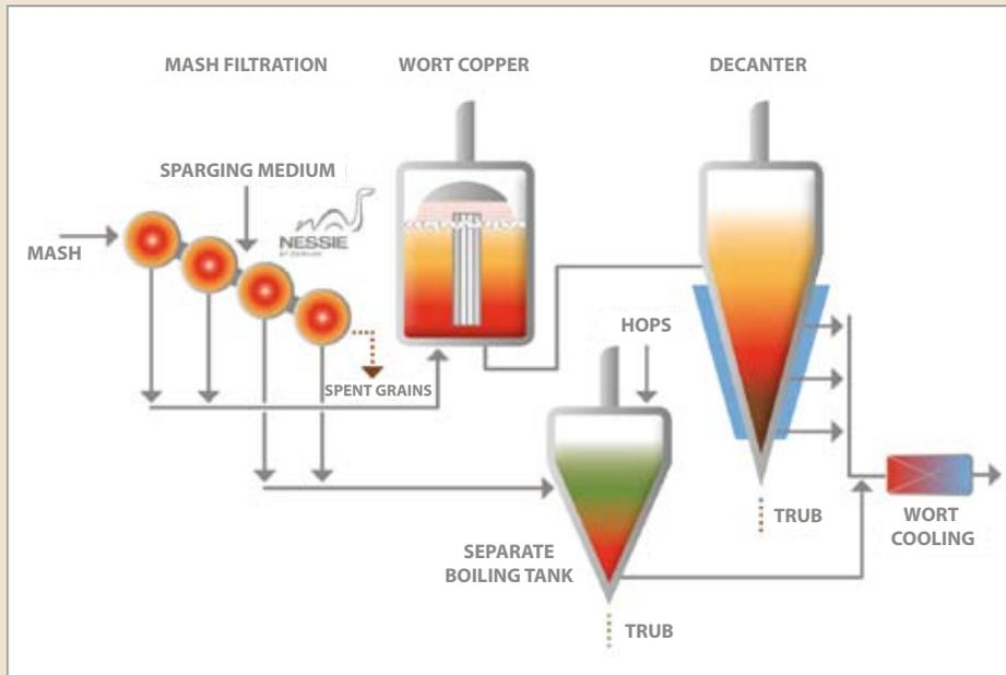
Fig. 4: Wort flow distribution of the novel mash filtration system for fractional wort boiling
